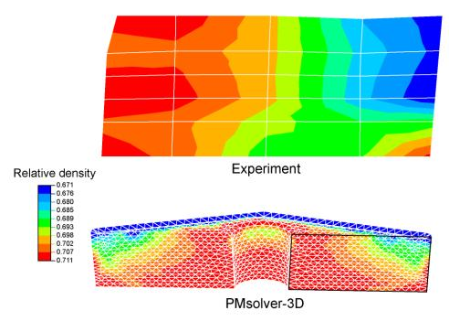
Figure 6. Comparison between the computer simulated green density gradients (PMsolver) and the experiment results taken from hardness tests on a cross-sectioned green compact of a cutting tool formed from WC-Co powder [35].
