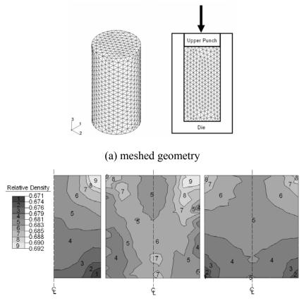
(b) result from experiment, explicit method, and implicit method Figure 10. Comparison of explicit and implicit methods for compaction simulation in the WC-Co system, where the half-axis experimental result is given on the left and the full-axis explicit method result is shown in the center and the implicit method result is on the right [35].
