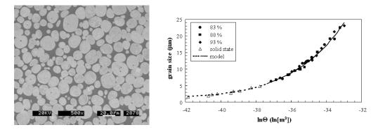
(a) SEM micrographs (b) grain growth modeling Figure 7. (a) A scanning electron micrograph of a liquid phase sintered tungsten heavy alloy (W - 8.4 wt.% Ni - 3.6 wt.% Fe) after quenching and (b) the grain size model results taken from an integral work of sintering concept that includes only the thermal cycle (timetemperature path) to predict grain size for any point in a heating path for three different tungsten contents [36].
