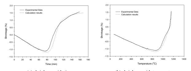
(a) shrinkage with time (b) shrinkage with temperature Figure 8. Dilatometry data showing *in situ* shrinkage data during constant heating rate experiments and the curve-fitting results used to obtain the material parameters to predict densification of a 316L stainless steel powder [38].
