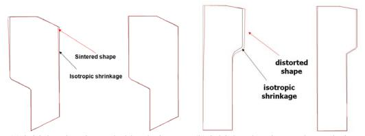
(a) initial and optimum holder designs (b) initial and optimum sleeve designs Figure 16. Final part profile files based on the combined press-sinter simulation for the optimized design of a holder and sleeve for an oxygen sensor.
