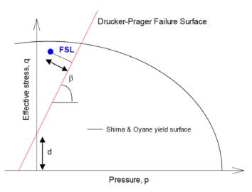
Figure 1. Definition of failure separation length (FSL) based on Shima and Oyane yield model and Drucker-Prager failure surface.
