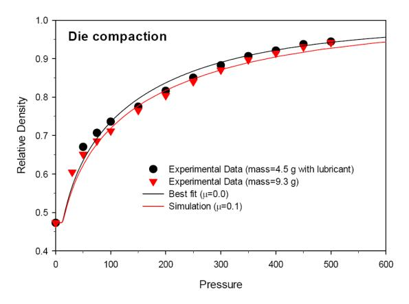
Figure 4. An example compaction curve for a iron-based powder, showing the relative density model results versus compaction pressure in MPa with no friction and with a friction coefficient of 0.1 for two compact samples [24].
