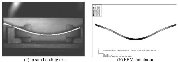
Figure 9. (a) A video image taken during the *In situ* bending test for a 316L stainless steel sample doped with 0.2 wt. % boron, and (b) the FEM model results used to verify the shear viscosity property as a function of time, temperature, grain size, and density during heating [39].
