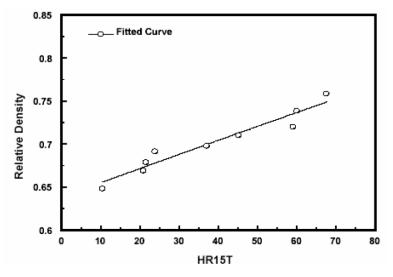
Figure 5. Plot of relative density and Rockwell 15T scale hardness for the die compaction of a WC-Co powder [35].
