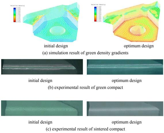
Figure 15. The effect of density distribution after die compaction on sintering and the formation of corner cracks.
